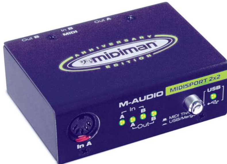
Figure 5-7: A basic MIDI interface with two Ins and two Outs.
